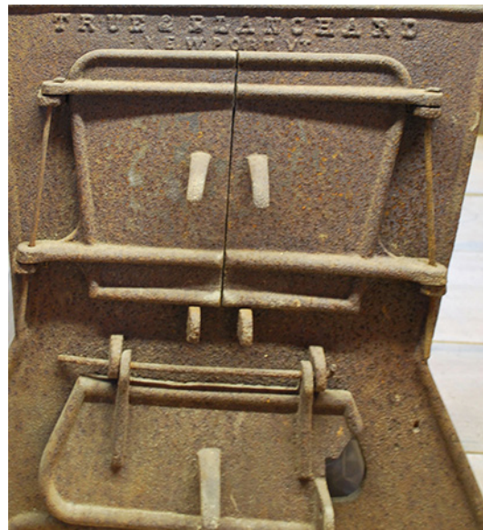
The fire door of the evaporator
